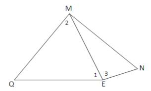
It is required to fix the co-ordinates of point Q from two existing beacons M & N. As it was impossible to set-up at point N, an eccentric station E was established near N so that the triangulation could be completed from M and E. Given:
