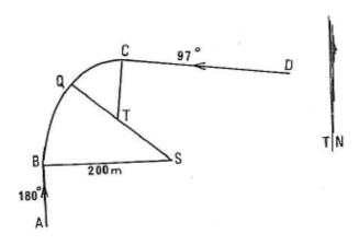
AB and CD are the centre lines of two straight stretches of a railway which are to be connected by means of a double curve BQC. BQ is the one and QC the other circular curve.
