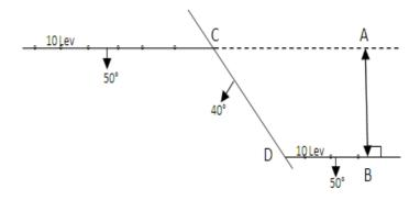
The plan shows two reef strike lines on the tenth level of a mine. A fault has dislocated the reef as shown on the plan.
