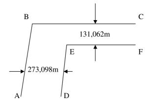
AB and BC form the Western and Northern boundary lines of a mine, B being the North – West corner.
